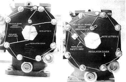
Note: The safety wire through the hex plug shown in the left hand photo is .025" wire wrapped around regulator screws under existing wire. It does not go through the holes in the screws. The safety wire through the hex plug shown in the right hand photo is .015" wire which passes through the regulator screw hole. This is the normal safety wire method used at the factory.
